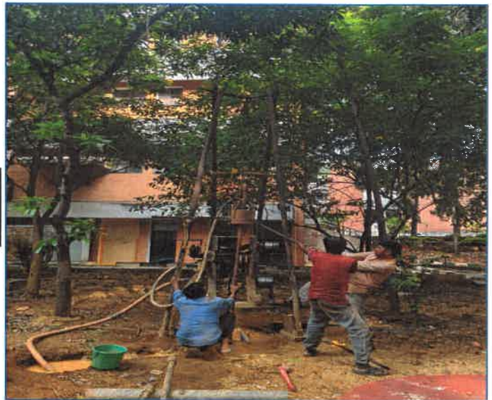
Standard Penetration Test in Progress
