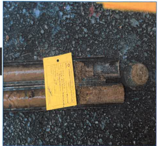
Soil Sample inside the Split Spoon Sampler
